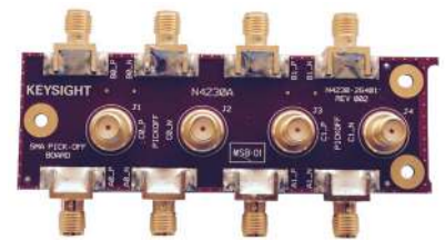
N4230A SMA breakout board for U4432A
