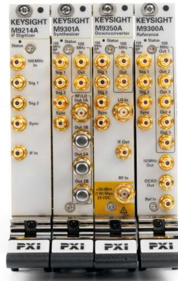
Figure 1. M9391A PXIe vector signal analyzer with four modules consisting of the M9214A digitizer, M9301A synthesizer, M9350A downconverter and M9300A frequency reference.
