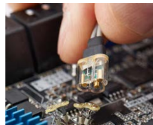
N2848A QuickTip head with N2849A QuickTip tips
