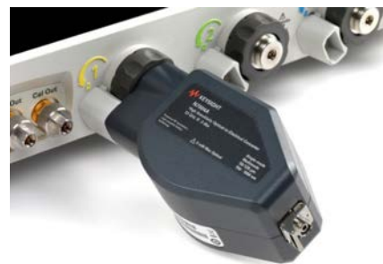
N7004A 33 GHz optical-to-electrical converter
