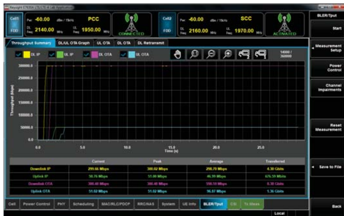
Figure 5. The UXM provides stable, bidirectional end-to-end data throughput
