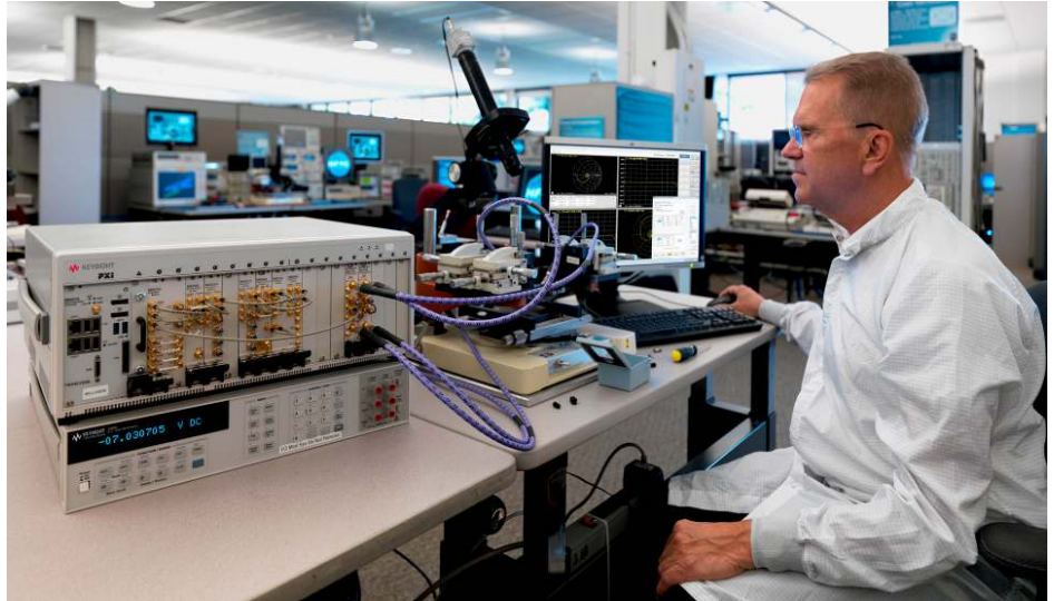
Figure 1. Using Keysight's M937xA PXIe vector network analyzer, M9381A PXIe vector signal generator and M9391A PXIe vector signal analyzer with measurement application software for power amplifier test.
