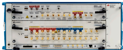
Figure 29. Overview of possible J-BERT M8020A configurations.
