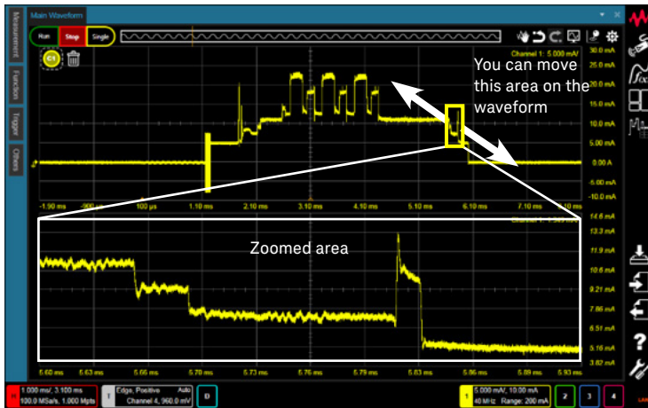
Figure 16. The “Anywhere” Zoom works like a magnifying lens on the waveform.
