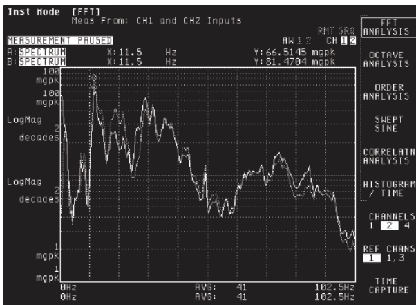
Two spectrums of road induced vibration measured at different speeds are compared using the front/back mode of the 35670A.
