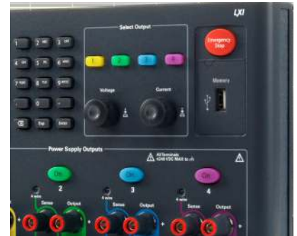
Figure 11. The N6705's front panel USB port.
