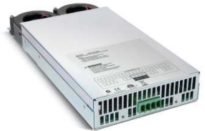
Figure 15. The N6750 high-performance series and N6760 precision series DC power modules that are \geq 300 W each occupy two modules slots within the mainframe. All other modules occupy one module slot.
