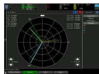
Phasor diagram for phase relationship analysis
