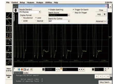
The PCI Express® electrical performance validation and compliance software lets you test devices to ensure compliance with the PCIe 1.1 and PCIe 2.0 electrical specs for add-in cards and motherboards.
