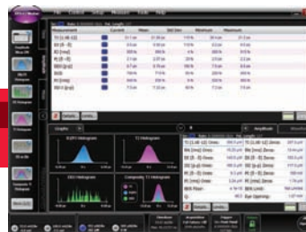
Advanced jitter and amplitude analysis. Accurate decomposition of impairments provides compliant total jitter (TJ) results and insight into root cause of eye closure.
